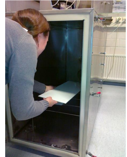
Photo: Testing chamber for determination of emissions to indoor air
