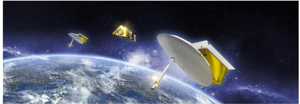
Space segment with two reflector satellites and one phased-array satellite
